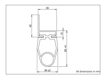
The Safety Edge meets the requirements for automatic reset, since after removing the operating force, it will return by itself into the ON condition.
